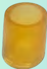
POLYURETHANE LARGE BUSH ID-54,ODBE-89.9,ODSE-67,L-111 SHORE - 50 to 70 (YSM 1373)
